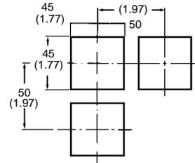
Note: Recommended panel thickness is 1 to 3.2 mm.
