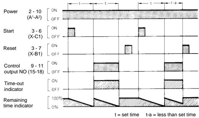
**Mode G Signal ON-delay/OFF-delay**
