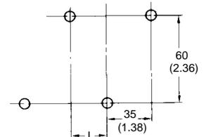
Note: When mounting two or more timers next to one another, allow 10 mm (0.39 in) between timers (dimension L).
