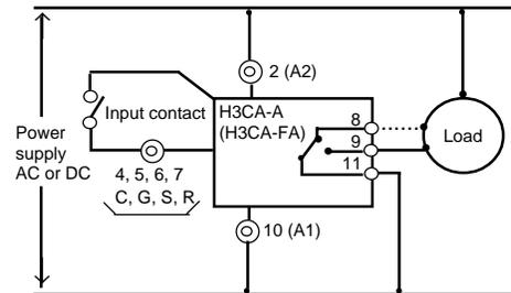
■ PROPER OUTPUT CONNECTIONS
