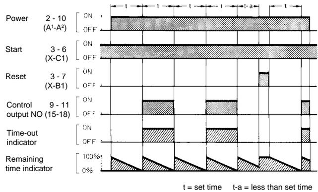
**Mode C Signal ON/OFF-Delay**
